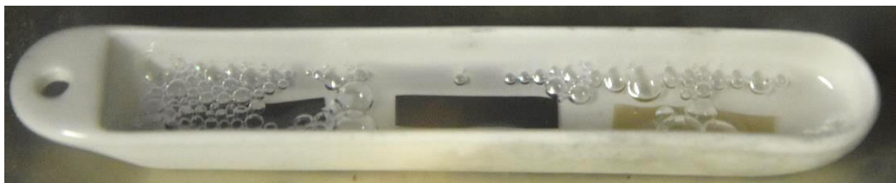
Figure 26. BNNT mats submersed in precursor and exposed to vacuum
