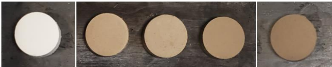
Figure 43. Pressed powder samples (0, 1, 5, 10, 20 wt%, respectively) before pyrolysis
