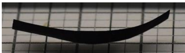
Figure 28. Side view of BNNT-SiCN sample (28 wt%) with initial manufacturing method
