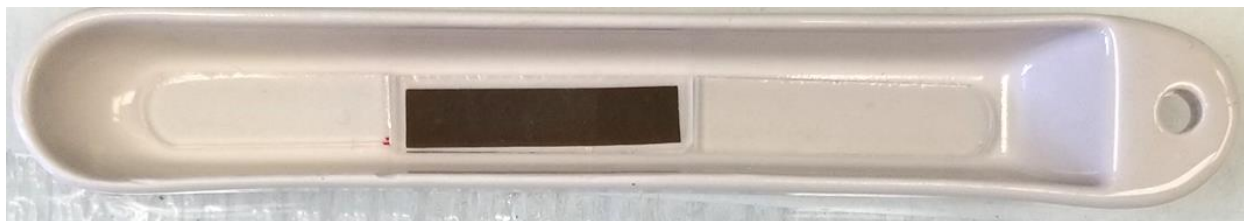
Figure 27. Quartz glass placed on top of composite mat to help prevent warping during heat treatment
