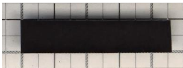
Figure 29. Top view of BNNT-SiCN sample (35 wt%) with improved manufacturing method
