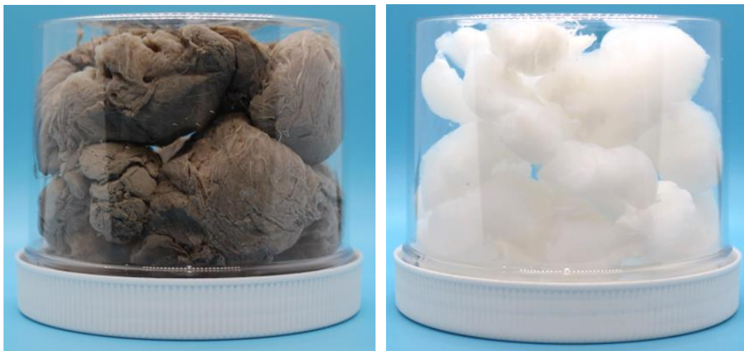
Figure 12. Puffball BNNT: raw (left) and refined (right) (from BNNT, LLC website)
