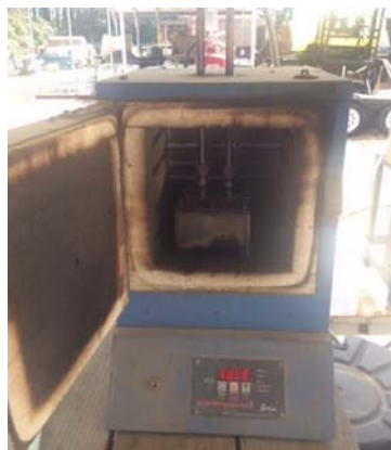
Figure 2.8 Muffle furnace containing the metal box container for heating the biomass
