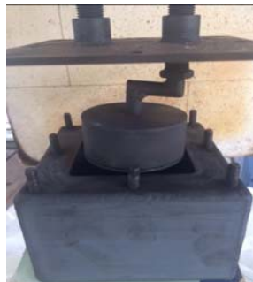
Figure 2.10 Metal tube attachment at the inlet to the metal container for distribution of the moist nitrogen mixture
