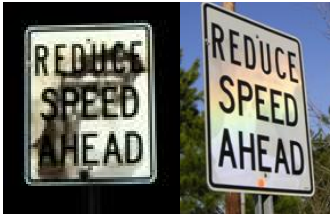
Figure 7.12. Night and Day Time Comparison of a Water Damaged Sign
