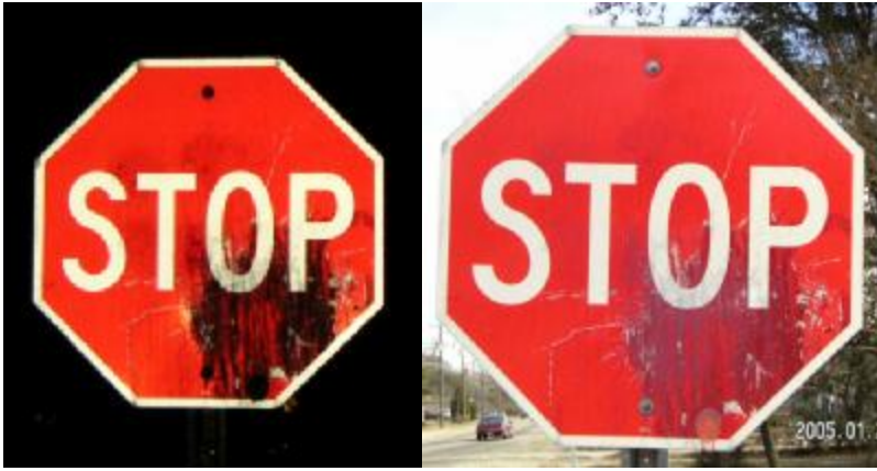
Figure 7.10. Night and Day Time Appearance of Sign with Paint
