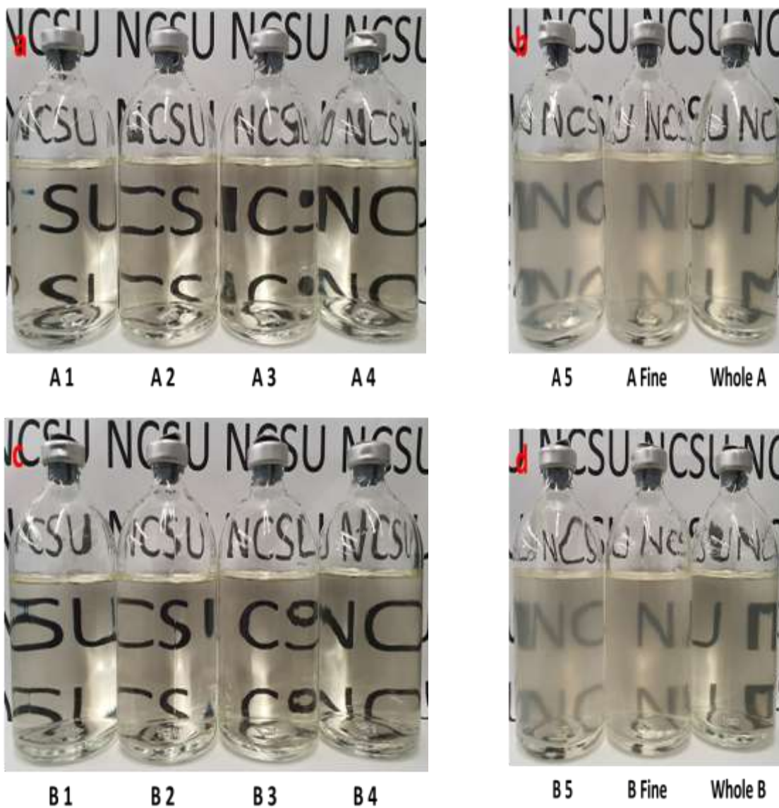
Figure S5.1. Two-step hydrolysate solutions produced from long fibers (left) and short fibers (right) of a and b cotton linter dissolving pulps A; c and d cotton linter dissolving pulp B, respectively
