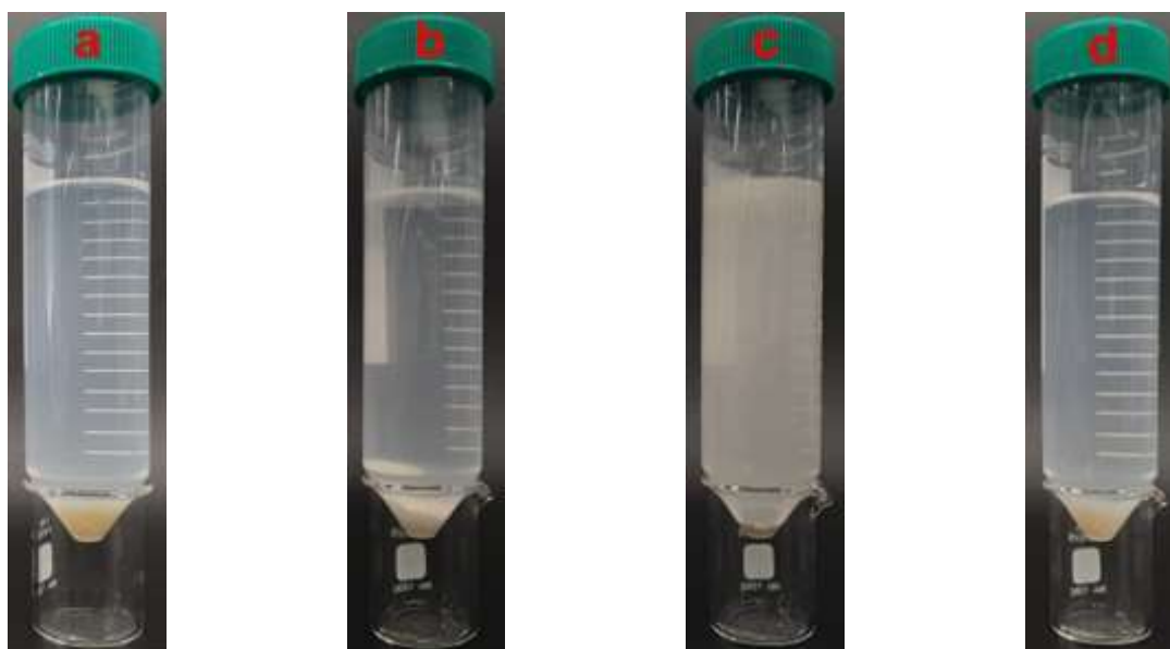
Figure 4.6. Photos of insoluble residue (a) collected after the demonstration of Type B IGP formation, (b) collected after acetylation and hydrolysis process, (c) collected from an experiment for investigating influences of the precipitation process, and (d) collected from an experiment for investigating influences of the drying process.
