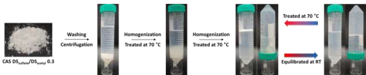
Figure 2.1. CAS hydrogel formation procedure and its thermal reversibility (Solid content: 4.5 wt. %)
