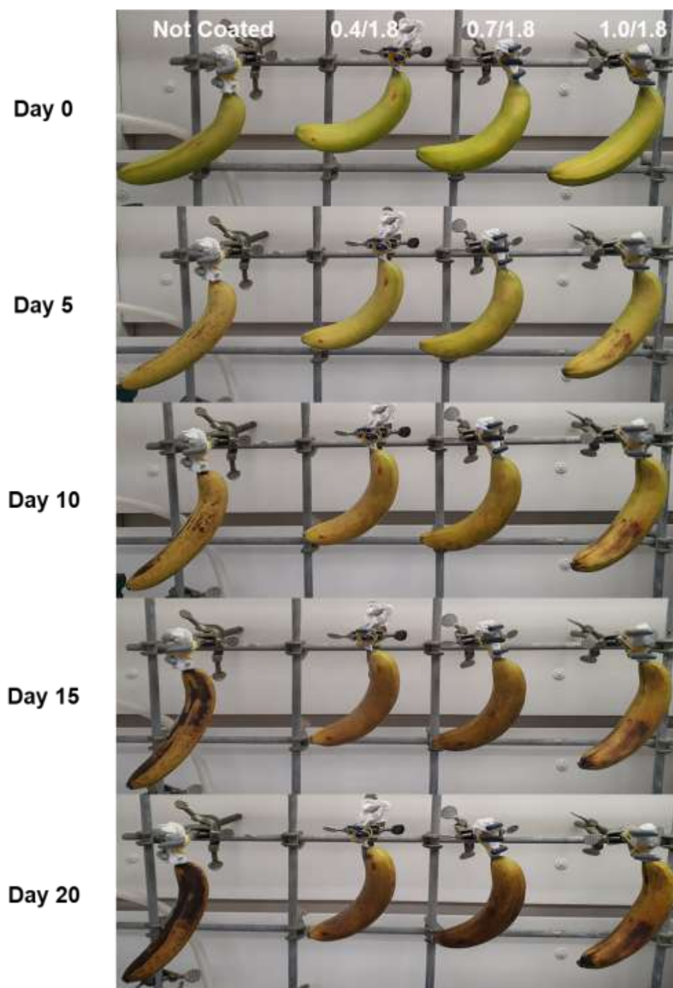
Figure 3.8. Comparative study of CAS coating using DS_{\text{sulfate}}/DS_{\text{acetyl}} 0.4/1.8, 0.7/1.8, and 1.0/1.8 film forming solutions.
