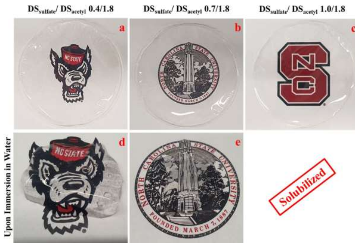
Figure 3.6. Photographs of (a) DS_{\text{sulfate}}/DS_{\text{acetyl}} \ 0.4/1.8 , (b) DS_{\text{sulfate}}/DS_{\text{acetyl}} \ 0.7/1.8 , (c) DS_{\text{sulfate}}/DS_{\text{acetyl}} \ 1.0/1.8 film, (d) DS_{\text{sulfate}}/DS_{\text{acetyl}} \ 0.4/1.8 film, and (e) DS_{\text{sulfate}}/DS_{\text{acetyl}} \ 0.7/1.8 film upon immersion in deionized water for 1 hour
