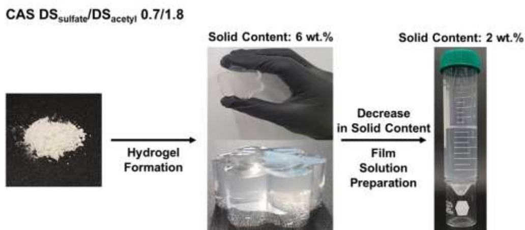
Figure 3.2. The procedure for preparing CAS film solutions
