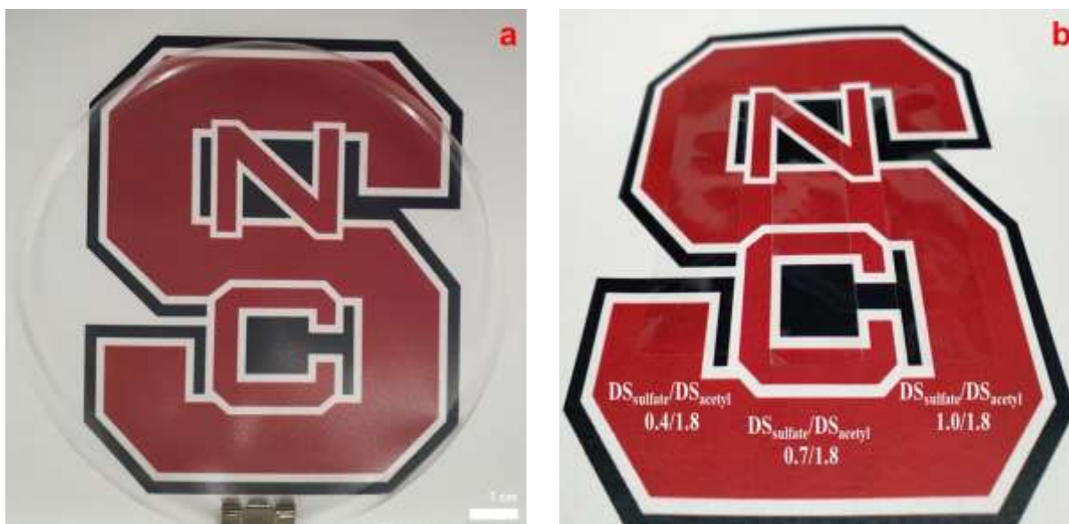
Figure 3.4. (a) A CAS film prepared from a CAS film solution with the DS_{\text{sulfate}}/DS_{\text{acetyl}} balance of 0.7/1.8 and (b) Three strips of CAS films made from different film solutions with varying the DS_{\text{sulfate}}/DS_{\text{acetyl}} balances (0.4/1.8, 0.7/1.8, and 1.0/1.8)
