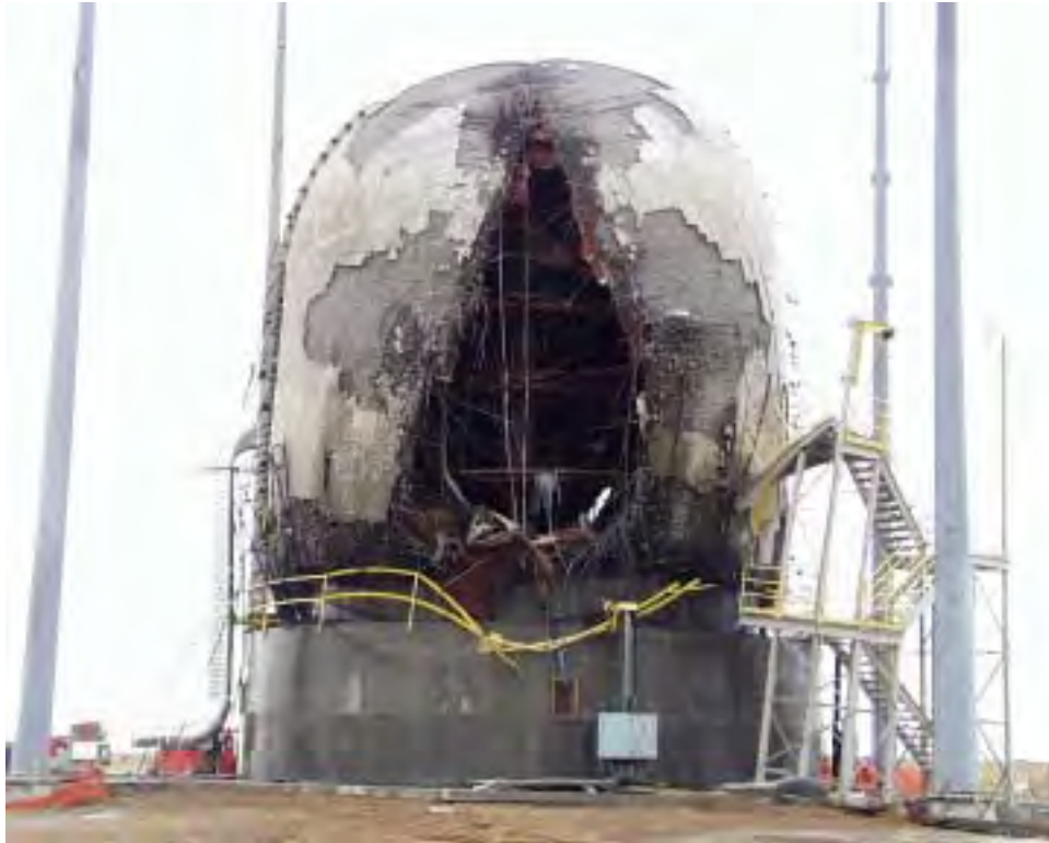
Figure 5. PCCV Model after the Structural Failure Mode Test
