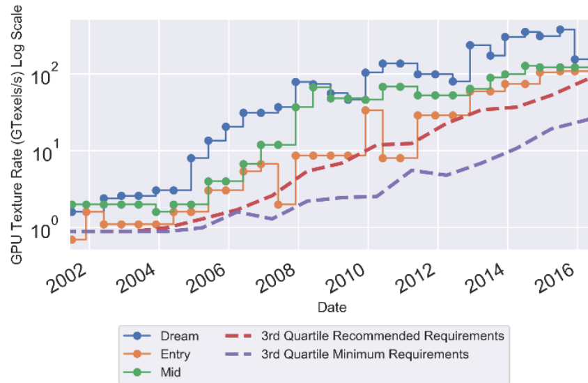
Figure 4.4: Suggested computer GPU performance vs Video Game Requirements showing desktop hardware increasingly outpacing game requirements beginning around 2005
