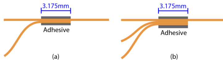
Figure 5.4 Sketch of the (a) 2x1 and (b) 3x1 acoustic coupler.
