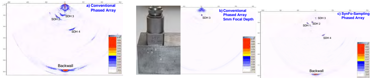
Figure 7: Near field characteristic of a conventional (left, middle) and the sampling phased array (right)
