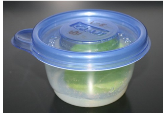
(b) Container used for bioassays in 2012. Containers were layered with 1% agar with leaf disc resting on top. © H.Alejandro Merchán
