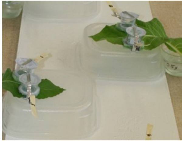
Figure A.6 Example of an experiment setup. Cages were constructed cutting about 5 cm from Falcon ® tubes, sealing one end with a metal washer and organdy mesh. Each cage was glued to one arm of a bent hair clip while another metal washer with a round piece of foam glued to it was affixed to the other arm. Extra foam was also glued to the open end of the cage to produce a tighter seal and to avoid damage to the leaf.
