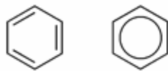
Figure 1.5 Structure of benzene showing (a) alternating \sigma and \pi bonds, and (b) delocalization of the three \pi bonds among the six carbon atoms
