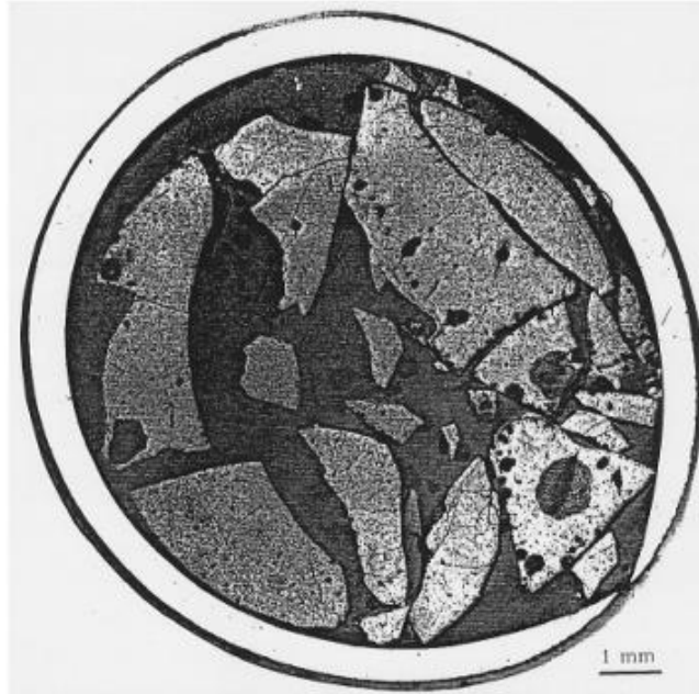
Figure 12: Fragmented fuel at rupture plane [19]
