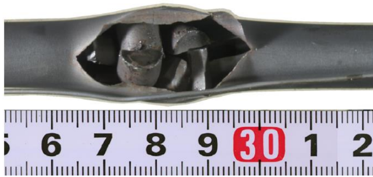
Figure 11: Ballooned region of cladding with relocation of fuel present [19]
