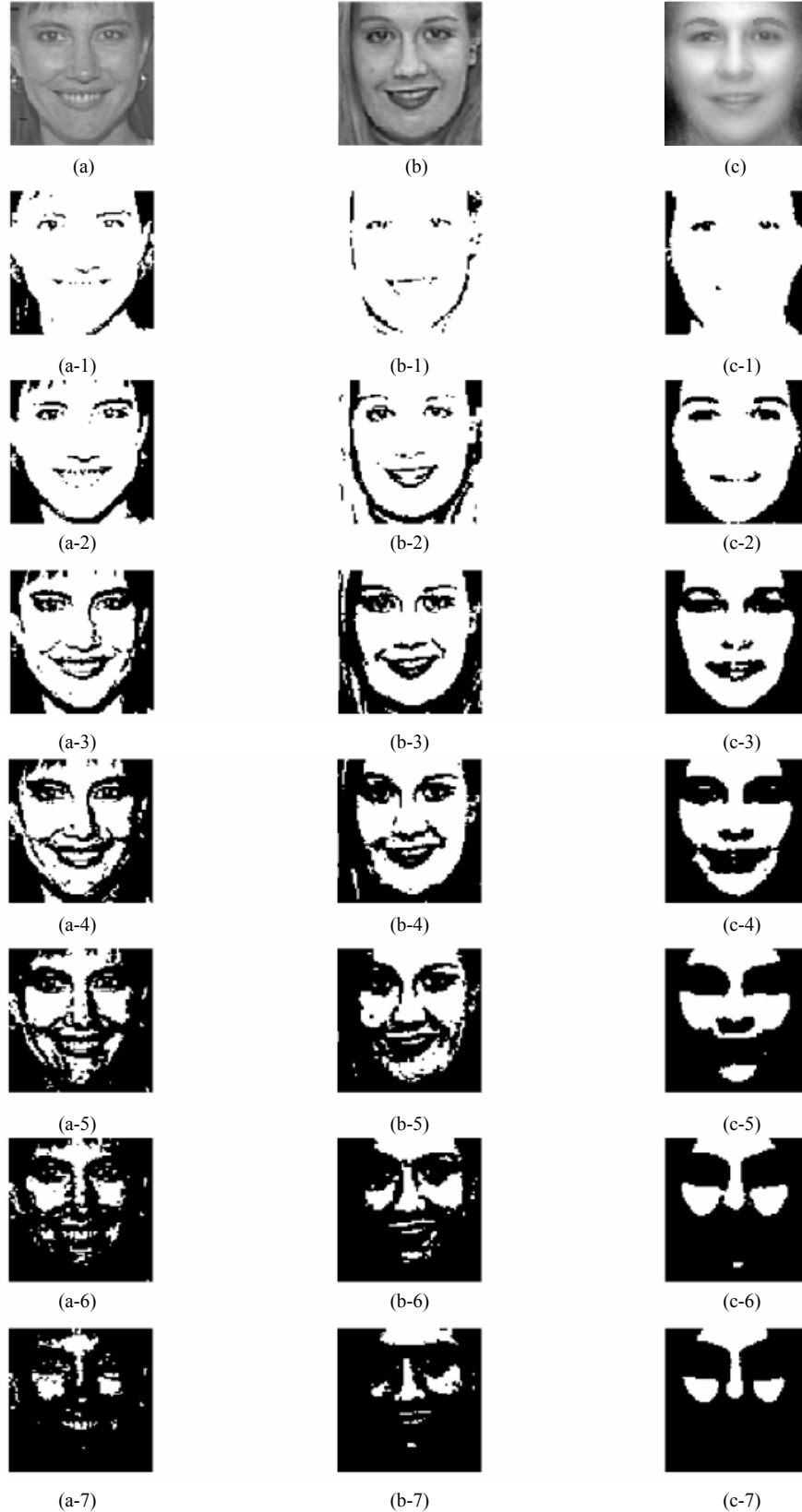
Figure 3.2: (a),(b) Examples of cropped database images, (c) the mean image; and their level sets, 1 through 7, in ascending order.
