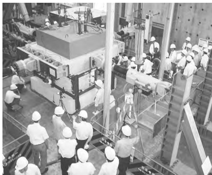
Fig. 4 A snap shot of the simultaneous Horizontal two directional loading test
