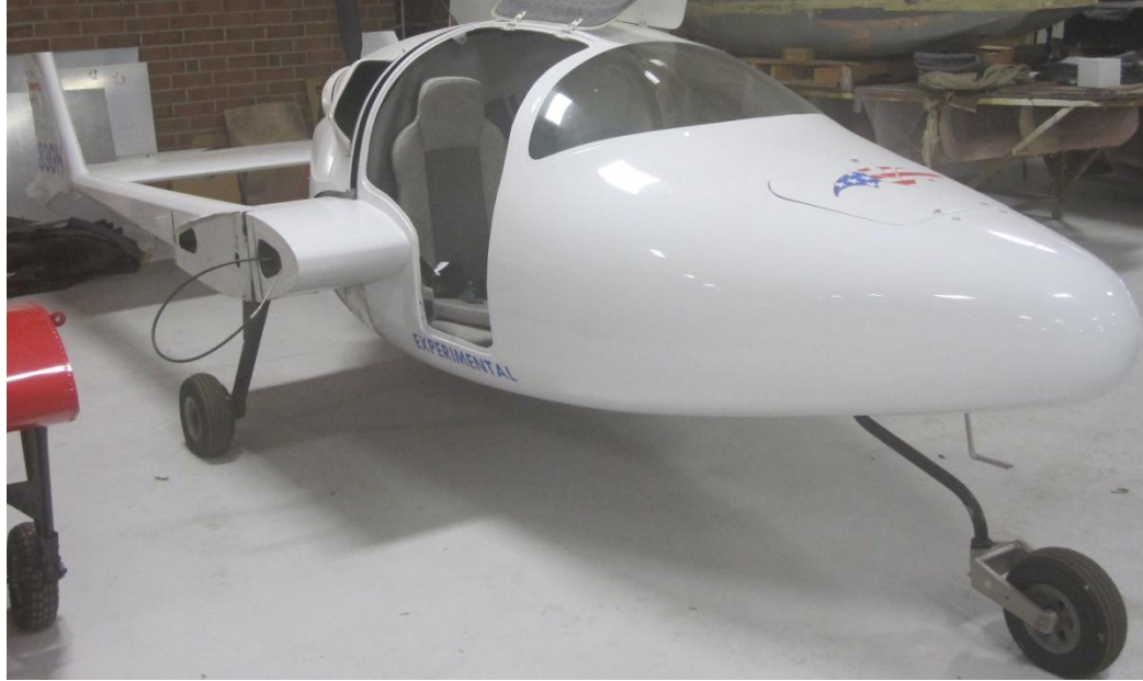
Figure 6: Vampire LSA. Note main gear inside tail-boom
