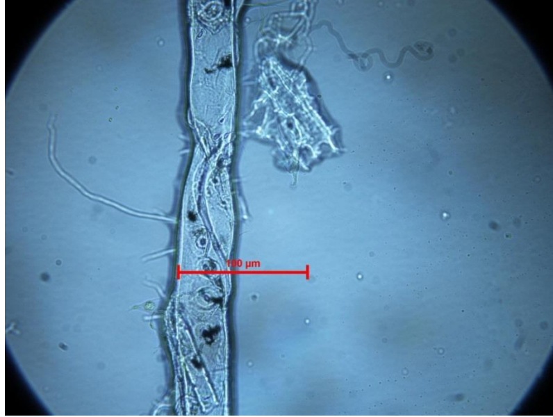
Fig. 5.4 Microscopic image of a representative newspaper softwood fiber, the length scale indicates 100 \mu\text{m}
