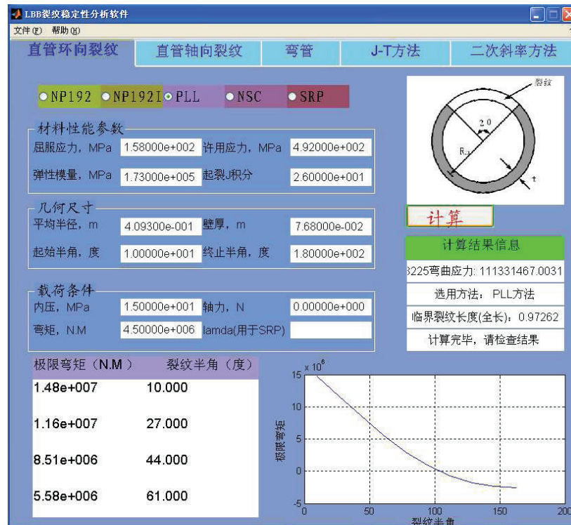
Figure 2 .The interface of LBB crack stability analysis code
