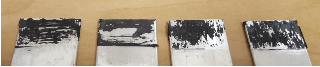
Figure 5.3: Images of the failure surface after shearing showing the cohesive failure. The two samples on the left had the CNTs oriented in the direction perpendicular to the strain and the two samples on the right had the CNTs oriented in the direction of strain.
