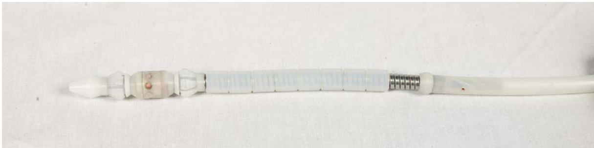
Fig.6: Array probe, INETEC ACV array probe with 8 cross-wound coils for VVER collector material examinations
