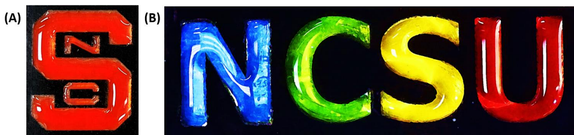
Figure 3.10 A) and B) Wettability contrast of NCSU pattern and logo; filled with hexadecane (red), water (blue), water + 4mm SDS (green), and water + 1mm SDS (yellow).
