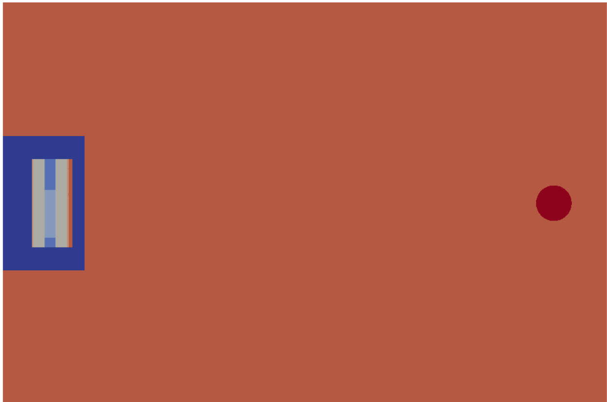
Figure 4.5: The simplified model of the shielded case as used in THOR. The view is a slice through the middle of both the BeRP ball and detector. Mesh boundaries are hidden.
