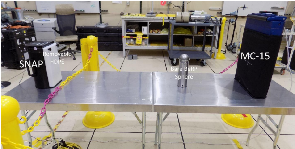
Figure 4.1: Experimental configuration of the BeRP ball and detectors on August 3, 2017. Copied here from Ref. [6].
