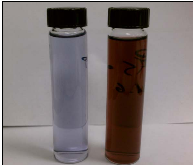
Figure 9.6 - Effect of Soda Ash Ending Dyebaths (L-no soda ash, R-with Soda Ash)
