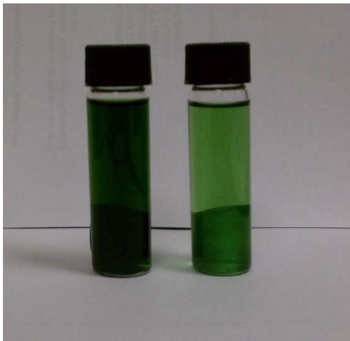
Figure 10.10 - Green Dyeings Boiled in Dibasic Sodium Phosphate (L-without soda ash, R-with soda ash in the dyeing)
