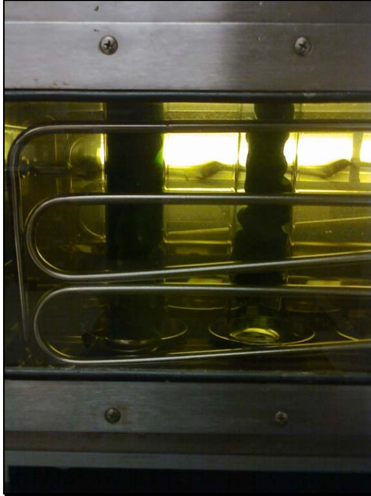
Figure 7.3 – Visual Observation of Effect of CMC (Left-with CMC, Right-no CMC)
